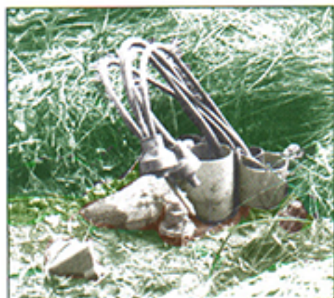
Most electrical connections undamaged. Enables reinstallation time and expense to be substantially reduced.
