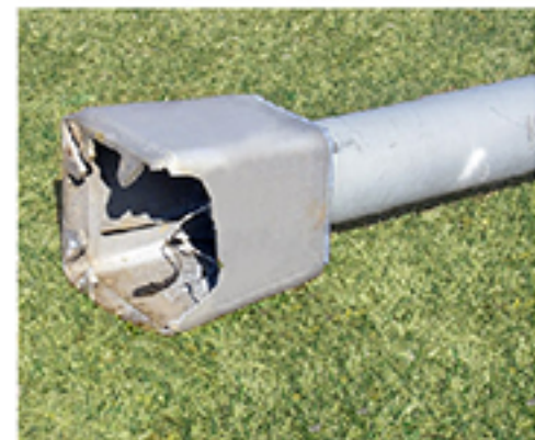
After impact, in most cases, pole is undamaged and can be remounted on a new transformer base.
