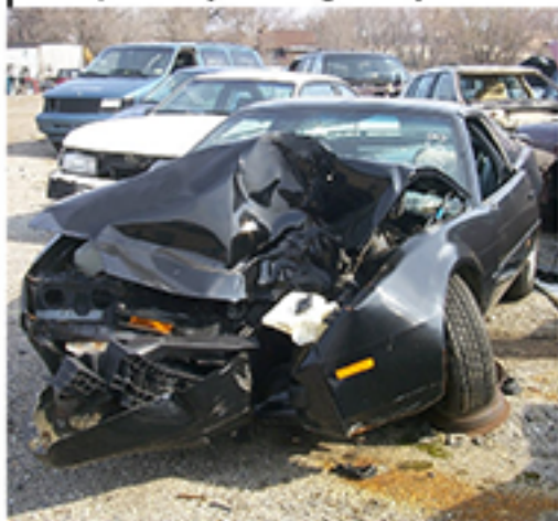
Severely damaged automobile after collision with a light pole not using a breakaway transformer base.
